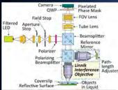
Microscope schematic for epi-illumination with a Linnik interference objective. Transparent samples in liquid are imaged in double-pass under a coverslip on a reflective surface. This system measures relative integrated optical thickness (OT) [or optical path difference (OPD)]. OT is proportional to physical thickness and index of refraction
